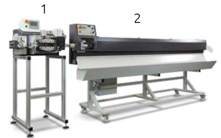
Inline assembly example: 1 Automatic cutting machine 2 Stacker
