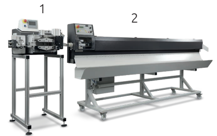
Inline assembly example: 1 Automatic cutting machine 2 Stacker
